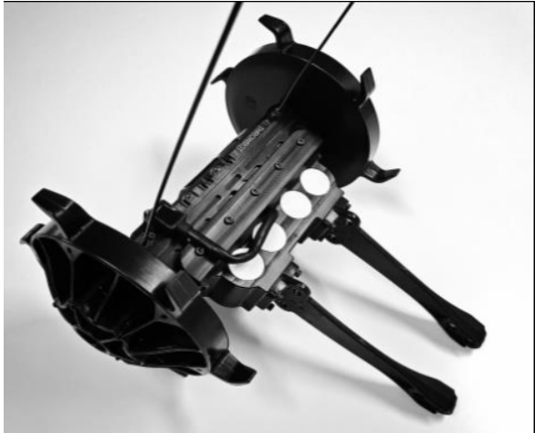
Figure 14: Integration of SARBI into the Throwbot2
